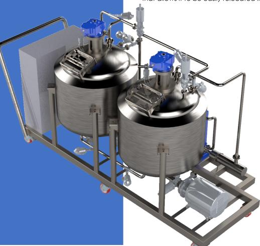
The tanks have a surface finish  $Ra \le 0.8 \mu m$  on all parts in contact with the product, clamp connections, and the main element, a vertical agitator with a three-bladed propeller and a sealing system by means of a mechanical seal.
